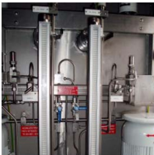
Fig. 6: Level gauge for the return and supply reservoir.
