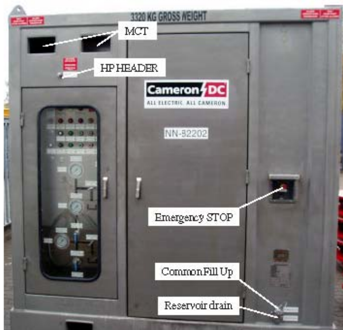
Fig. 8: Front of the K5F-HPU with hydraulic connections.
