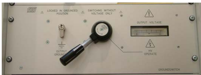
Figure: Groundswitch with its lock
