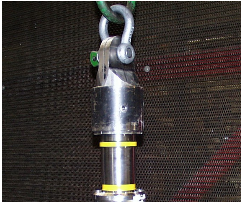
Photo: PRCM mandrel in UNLOCKED position, hanging from a crane secured by lifting eye PN 223260-99
