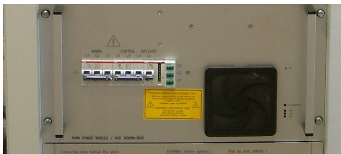
Figure: Fuses on front panel lower section
