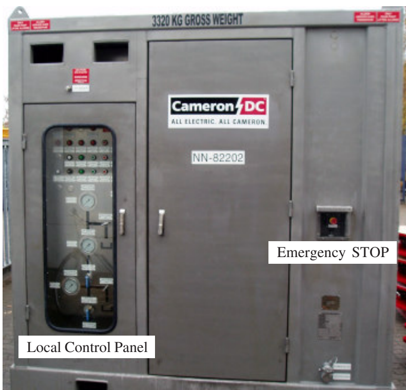
Fig. 2: K5F-HPU with Local Control Panel and Emergency STOP button.
